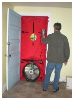
Testing the Blue House for air leakage
